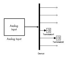
Depending on the board and the number of channels used, I/O conversion time can affect the maximum sample rate that can be achieved on your system. Rather than converting unused channels, we recommend specifying only the set of channels that are actually needed for your model.
